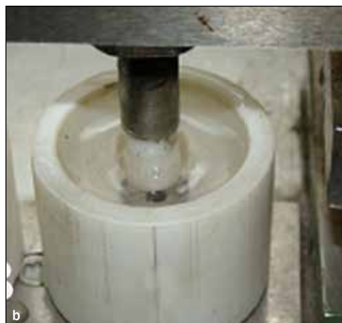
Fig 5 (a) The polyacetal tip manufactured for testing. (b) The piston contact with the specimen, which was immersed in saline solution at a temperature of 37°C.
