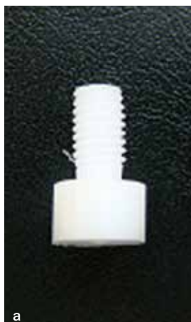
Fig 5 (a) The polyacetal tip manufactured for testing. (b) The piston contact with the specimen, which was immersed in saline solution at a temperature of 37°C.
