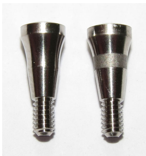
Figure 2 Healing abutments with a smooth surface and with a 1-mm transmucosal region with surface treatment, respectively.
