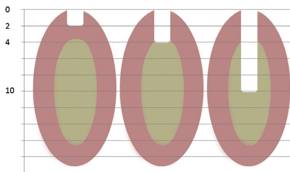
Fig. 3. Diagram of the sequence of intermittent milling depths.
