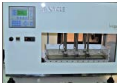
Fig 3 (Right) Image showing the samples immersed in water at 37^{\circ}\text{C} \pm 2^{\circ}\text{C} and placed on a mechanical cycler with the Biocycle machine.
