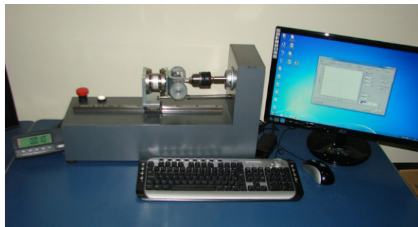
Fig. 2. Image of the computerized torque machine used in the removal torque test.
