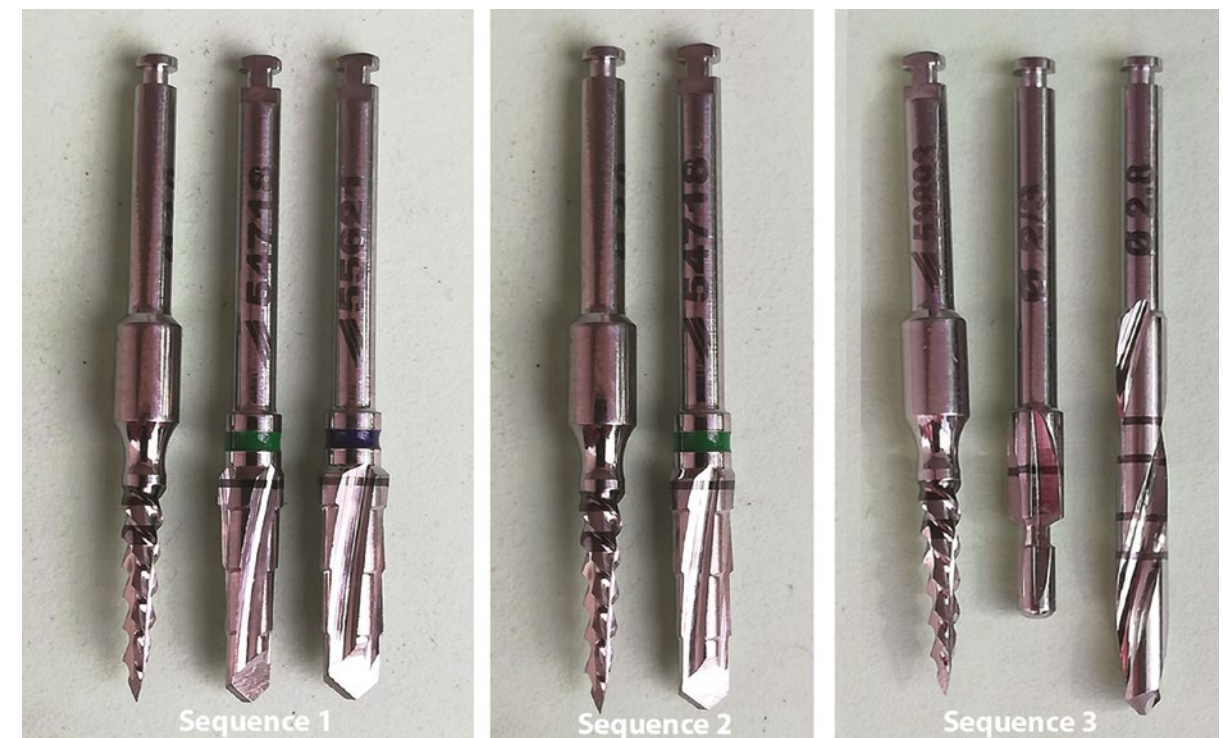
Figure 2: Image of the three drill sequences used to perform the osteotomies
